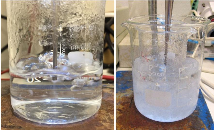
**FIGURE 3** Left: The Sonotrode placed in the middle of the cylinder, at a depth of 10 mm. Bubble ensemble underneath the Sonotrode during cavitation. This figure is an illustration photo to show the setup without obscuring the sample and Sonotrode from the ice cooling. Right: Beaker placed in ice-filled container. Parafilm removed for illustration purposes. Photos: SINTEF
