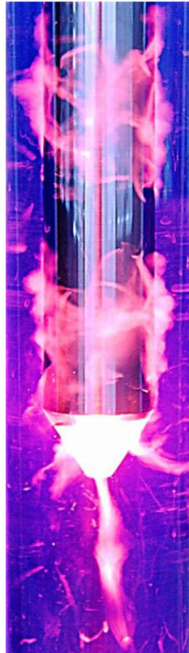
**FIGURE 2** Example image of cavitation around Sonotrode. Photo: Hielscher, Germany, ©www.hielscher.com, 2016
